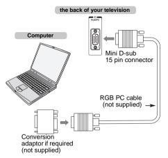
To use a PC, set the monitor output resolution on the PC before connecting it to the television. For acceptable PC signal formats, see page 87.
